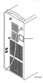
Check that the unit is connected to the correct mains power supply voltage, and that it is protected by the correct fuse sizes. A protective earth connection must be made, in accordance with regulations.
